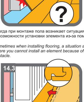
It's necessary to leave an installation and deformation clearance: not less than 10 mm from the edge of covering to the walls. Installation of laminate flooring should be started from laying of the 1st row. Plates are jointed by the edge at the angle of 15 degrees.
